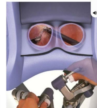
Fig. 71.5 The da Vinci Robotic Surgical System: stereo viewer that creates a virtual three-dimensional stereoscopic image. (Courtesy Intuitive Surgical, Sunnyvale, CA, USA)
