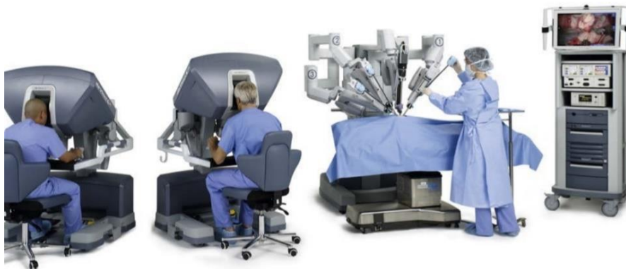
2 The da Vinci Robotic Surgical System: two surgical consoles, patient-side cart with four mounted surgical arms, and an optical tower. (Courtesy Intuitive Surgical, Sunnyvale, CA, USA)
