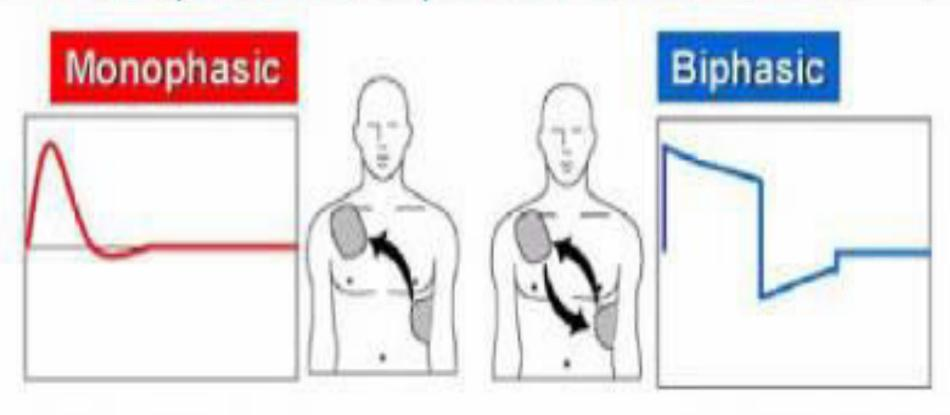
Current delivered in one direction Current delivered in two directions
